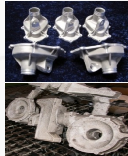
Aluminum -Castings AlSi7Mg
