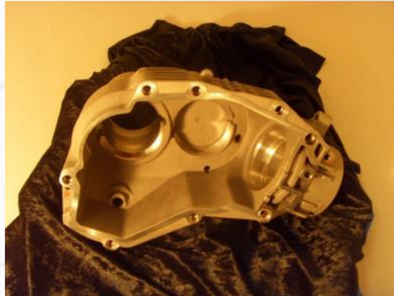
Compact casting Production time: about 16 working days
